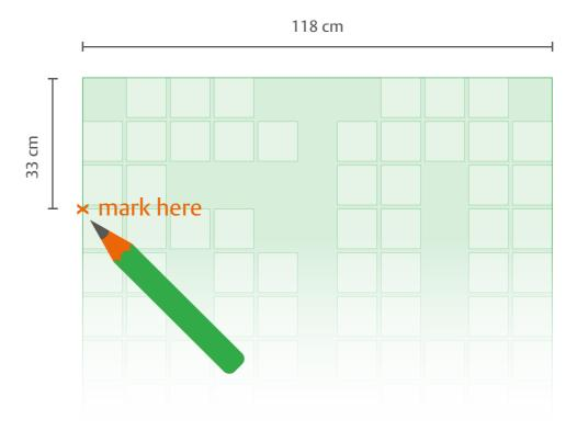
The small dot you have marked is the starting point. Take the spirit level and a portrait tile. Remove the tape from the back of the tile. Position the tile so that it is level, with the top left of the tile on the mark.
